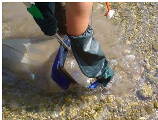
Figure 16: The substrate should be disturbed with a screwdriver or similar tool up to a depth of about 15 to 20 cm
