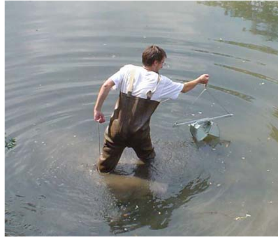
Figure 18: Van Veen grab, operated from a wadeable area near the bank
