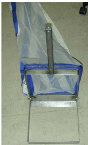
Figure 2: AQEM/STAR net sampler, with frame in front
