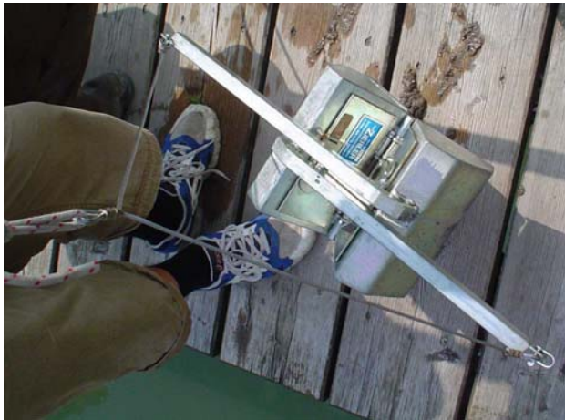
Figure 6: Van Veen grab, top view, open
