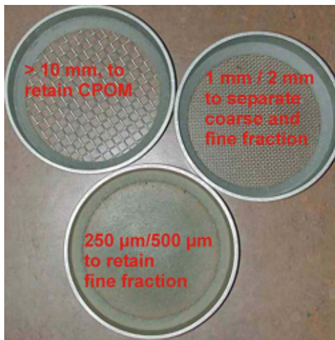
Figure 2: Set of sieves to be used for separating the coarse and the fine fraction
