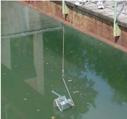
Figure 17: Van Veen grab, lowered down from a footbridge
