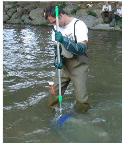
Figure 3: The net is held vertically with the frame at right angles to the current, downstream from your feet
