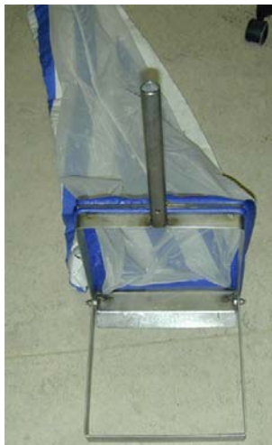
Figure 2: AQEM / STAR / ASSESS-HKH net sampler, with frame in front
